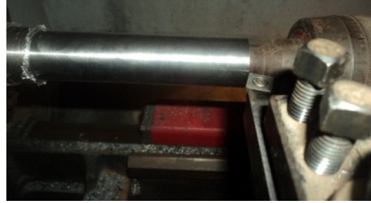
Figure 1 Photograph of experimental setup for turning Nimonic C-263
